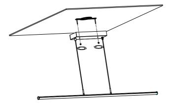
A-C: Secure the power box with screw nuts
