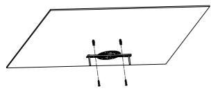
A-A: Screw the crossbar onto the wall by using self -tapping screws and Nylon Plug
