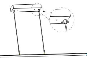
A-B: Attached the canopy to the crossbar and get the claer cable wired with AC input. The length of clear cable can be adjusted after loose the gripper in white
